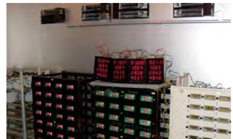
Burn-In at 55°C to Ensure Stability
