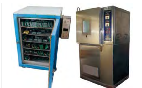
Enviromental Chamber To Simulate -20°C to 100°C (Rh upto 100%)
